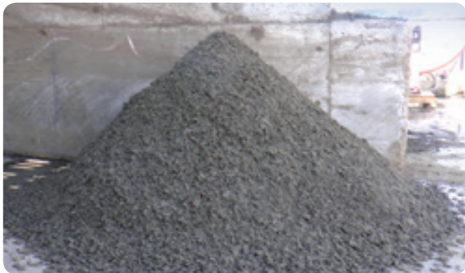
Fig 1. Solids from the Z-Filter discharged into a pile.
